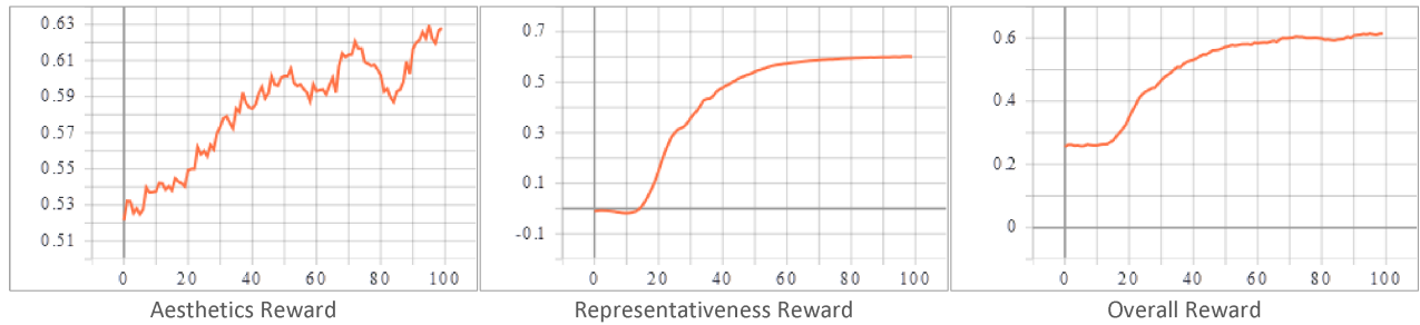
Figure 3: Reward curves for the proposed model. The horizontal axis in all plots indicates the epoch number. These curves show smooth training of the model, and the ability of the Thumbnail Selector to get higher rewards as the training proceeds.
